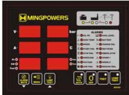
Control module Turkey Datakom 507
